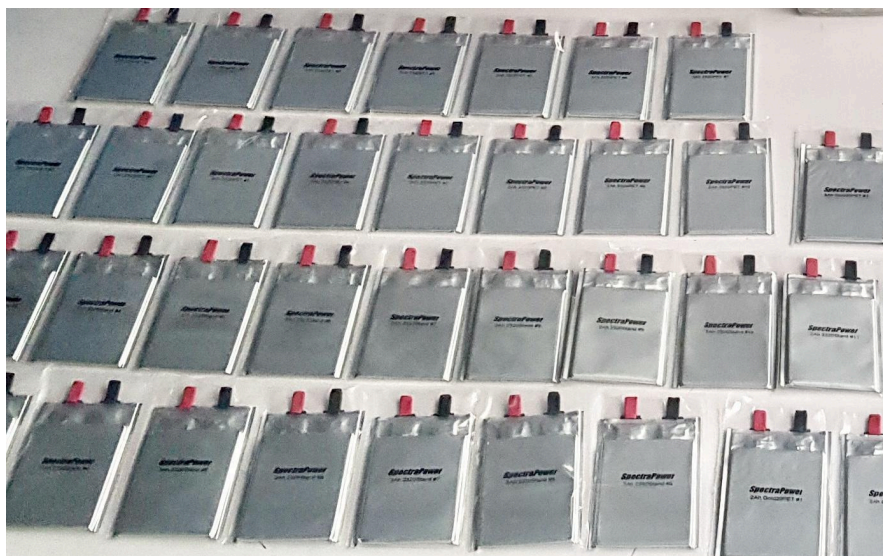
[FIGURE 2 – Example Multilayer Pouch Cell Builds]
